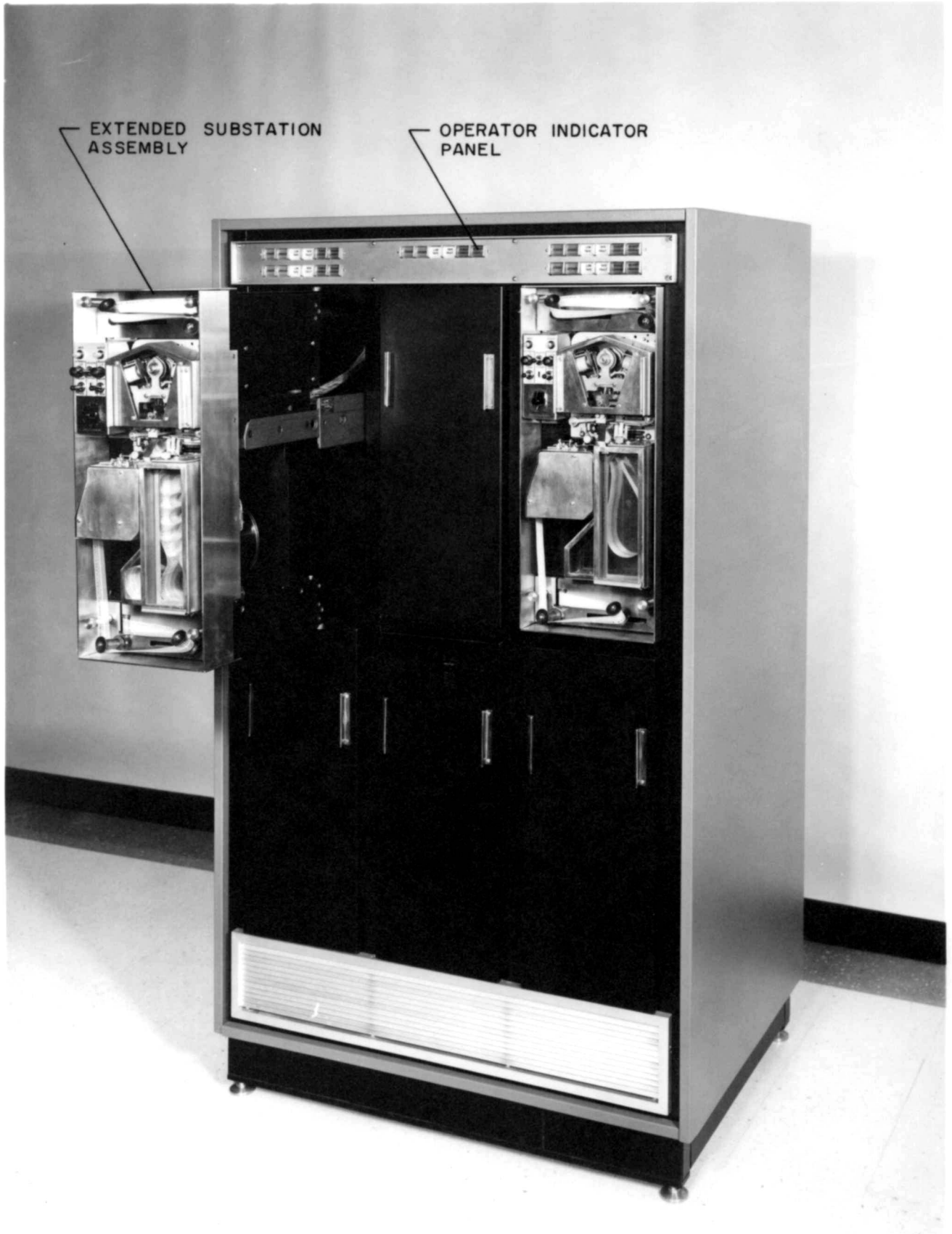
Figure 1-6. Substation Cabinet With One Substation Assembly Extended
